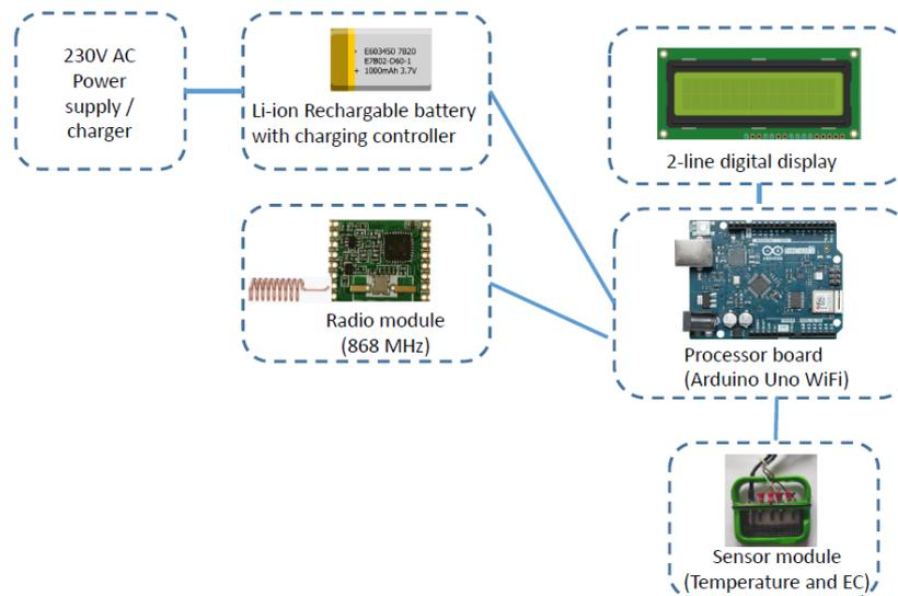
Fig. 1. Flowchart of IoT based prototype
